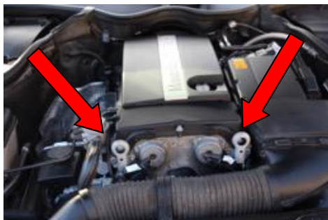
Cam position sensors and harness after Mercedes Benz campaign mod. Harness is now isolated
